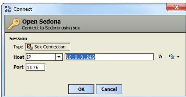
For the Sedona device we will use a controller in the BAScontrol series (BASC). Like other Sedona devices, the BASC is IP-based so we need Workbench to be on the same sub-net as the BASC. In this example we have the BASC addressed at 10.0.0.249. Using a web browser, we can try to access this IP address. If we obtain an Authentication Request from this controller, we are assured we are on the right sub-net. We can enter credentials for this controller to view the main
