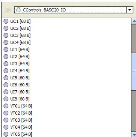
Using the drop-down, select the *CControls\_BASC20\_IO* kit. In the case of the BAScontrol20 there are 49 components to choose from – 20 real points, 24 virtual points, a scan timer and 4 retentive universal counters. All are intended for one time use and only those dragged onto the wire sheet will become part of the logic of the controller.
